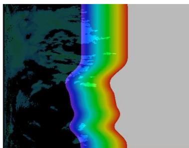
Figure 2. Reflectivity scan (rays clockwise top-to-bottom, bins left-to-right) from a radar with 460 km range, overlaid with quality indicator representing probability of overshooting.
