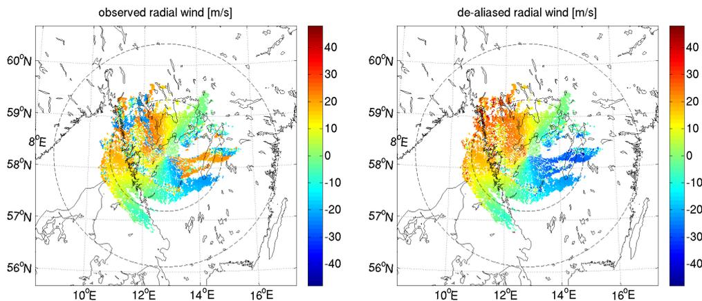
Fig. 6. Observed and de-aliased radial wind. The dashed lines indicate the 120-km and 240-km-range ring, respectively.
