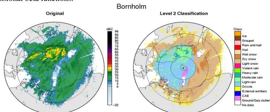
Fig. 5. The original radar image (on the left) and its corresponding level 2 hydrometeor classification (on the right).
