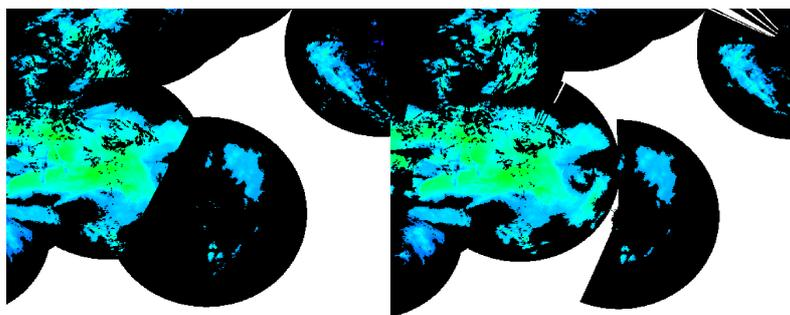
Figure 1. Detail from two experimental composites, one that hasn't been quality-controlled for beam blockage (left) and one that has been controlled (right). The corrected composite succeeds in capturing the precipitation that is blocked in the uncorrected composite.
