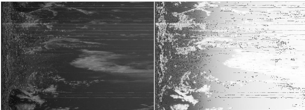
Fig. 4. Original sweep (on the left) and quality field (on the right) based on biometeor, emitter, ship, and speckle detections computed by AnDRe module of Rack.
