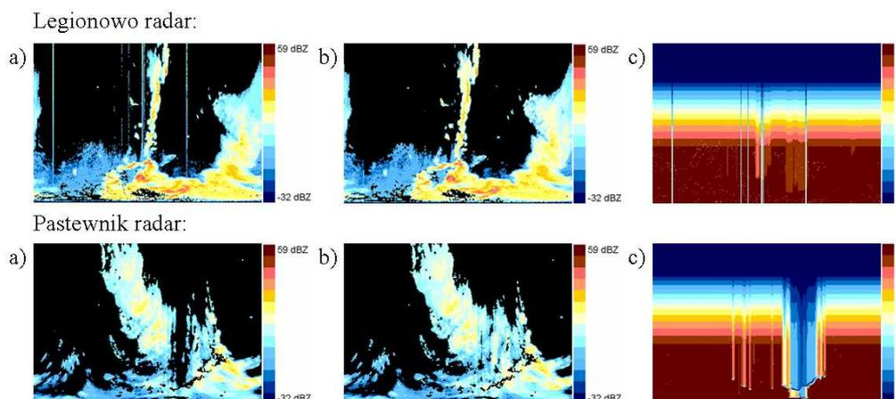
Fig. 3. Example of performance of all correction algorithms for the elevation (0.5°): a) raw data (in dBZ); b) corrected data; c) total quality index QI. Radar range is 250 km. The panels represent range (y-axis) vs. azimuth (x-axis) displays.
