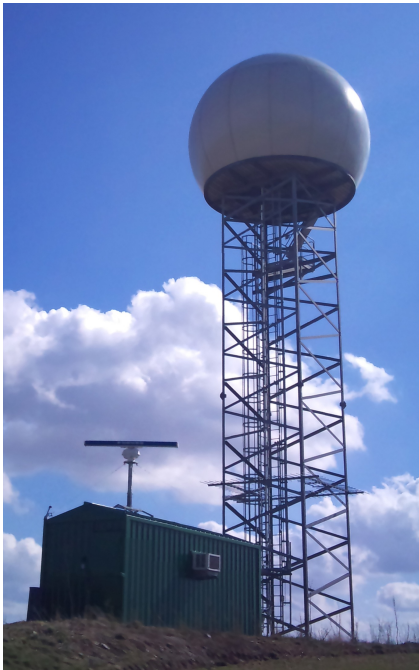
Figure 2. Direct comparison between the LAWR X-band radar and the DMI Dualpol C-band radar at Virring near Aarhus, Denmark
