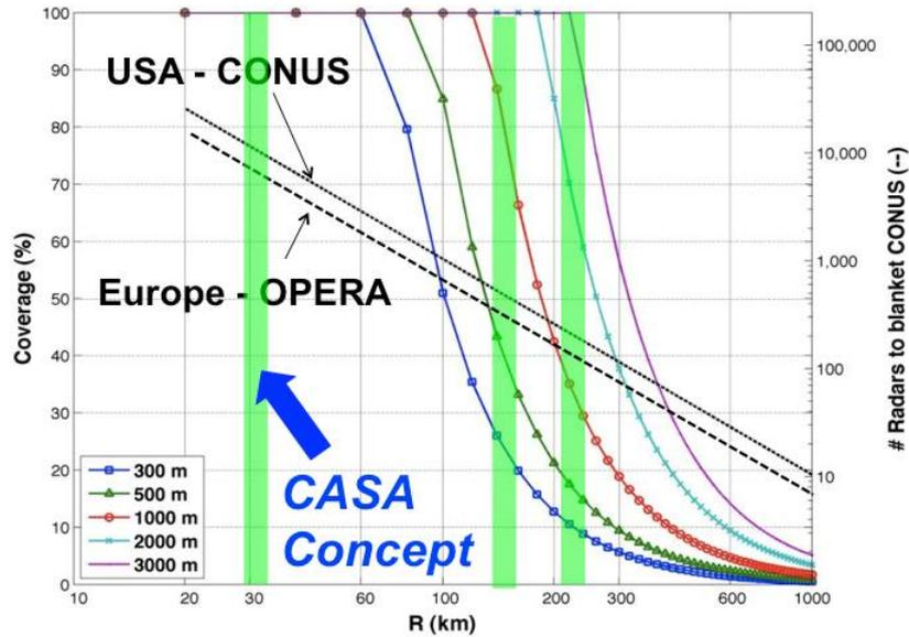
Figure 1: Percent coverage (solid lines) and number of radars needed for coverage over the continuous USA and European Opera region (dashed lines) vs. radar spacing.
