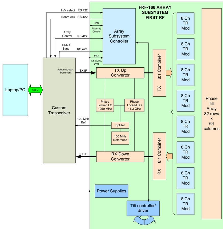
Figure 3: Phase-Tilt Weather Radar system block diagram.
