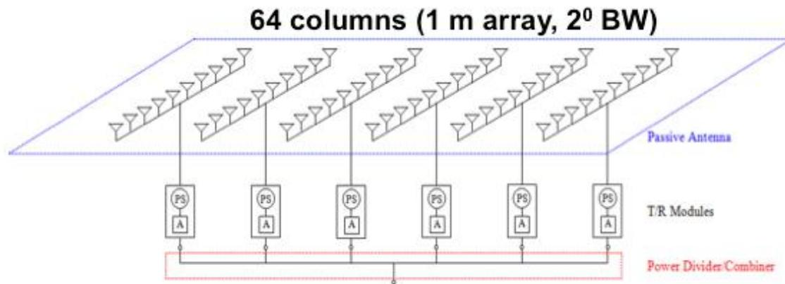
Figure 2: Schematic concept of phase-tilt antenna array.
