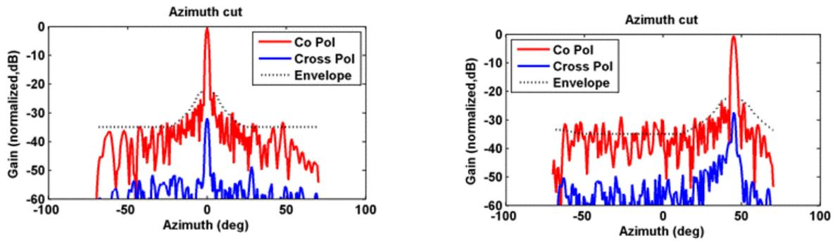
Figure 4: V-polarization azimuth cuts at  $0^\circ$  (left) and  $45^\circ$  (right), showing co- and cross-polarization performance
