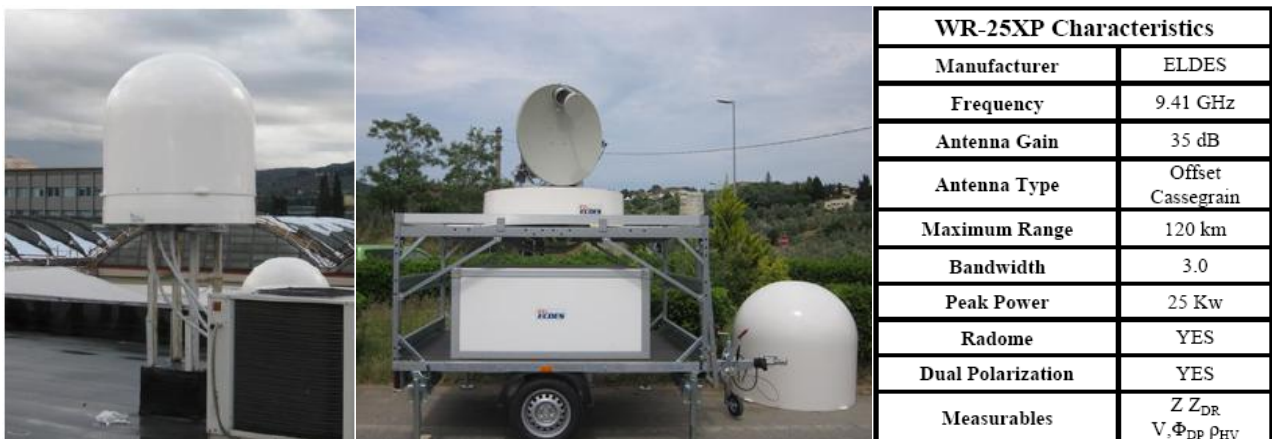
Fig. 1 Fixed WR-25XP radar (left) mobile unit (centre) and main operational characteristics (right)
