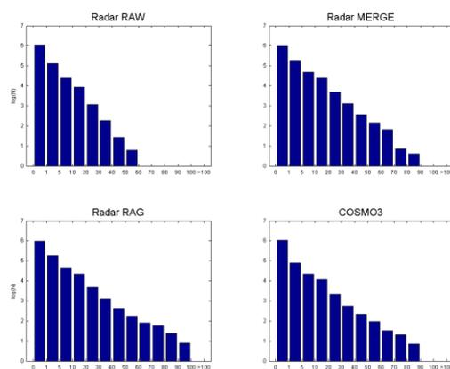
Fig. 1 The distribution of grid-point 3h precipitation over the verification domain and for all days of the convective period. The subpanels show raw radar precipitation (Radar RAW), the adjusted QPE values for MERGE (Radar MERGE) and RAG (Radar RAG) and for the rainfall predicted by COSMO 2.8km (COSMO3). Vertical axis show the number of rainfall values in logarithmic scale, horizontal axis indicates the 3h rainfall values.
