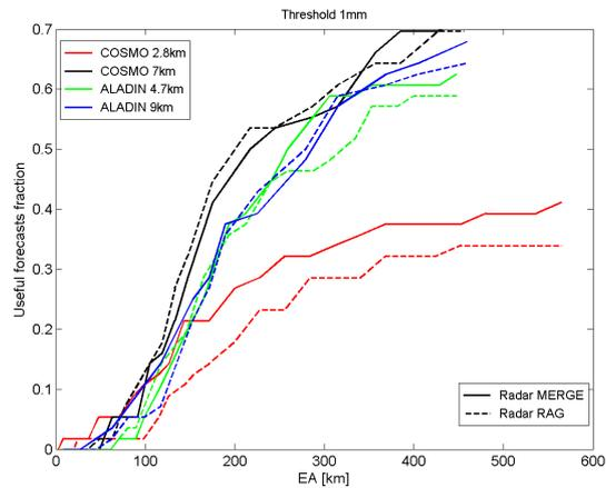
Fig. 3 Fraction of forecasts with FSS values larger than  $FSS_{uniform}$  for the precipitation threshold 1mm/3h. Horizontal axis represents the EA size in kilometers. The models and adjustment techniques are indicated in the legends.
