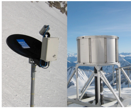
Fig. 1: Micro Rain Radar 2 (MRR) (left) and MIRA35 cloud radar (right) at the UFS Schneefernerhaus.
