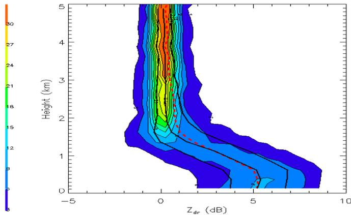
As opposed to S band,  $Z_{DR}$  at C band is very high in melting hail mixed with rain
