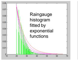
The chosen distributions were used as inputs to the PMM algorithm, which was modified to take account of the variability between the radar and raingauge values, and which is used to calculate adjustment factors for the radar rainfall data (right hand panel.
