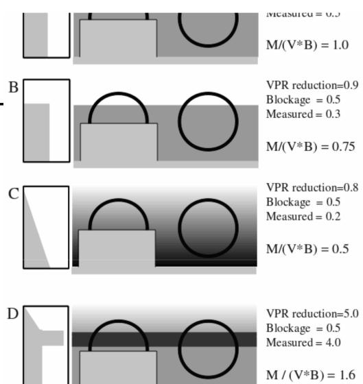
4 profiles of reflectivity (left) as seen by a beam that is 50% blocked (centre) or unblocked (right). The results of multiplicative correction to 50% blockage case are shown on right.
