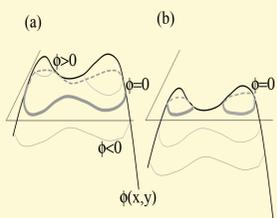
Evolution of the  $\phi$  function during a splitting event. The heavy grey line stands for the object contour. (a): One object is present. (b) two objects appear.
