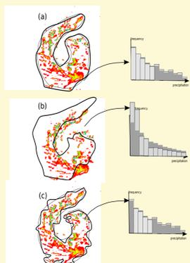
(a): Two slightly different objects with comparable frequency histograms. (b): objet whose shape is comparable with (a) but with significant space shift. The corresponding histogram is now different from the original one with an excess of weak precipitation. (c) here two objects with close histograms but with different level of smoothness.
