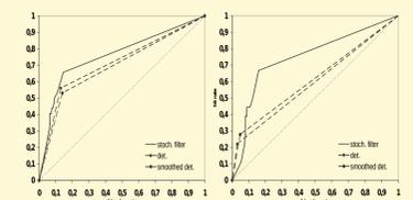
ROC curves along the time integration of the filter. The event to be detected is associated to precipitation intensity of 0.3 mm/h (left panel) or 1 mm/h (right panel). Deterministic forecast based on direct model outputs, resp. smoothed ones, are denoted by dashed lines and squares, resp. black bullets.
