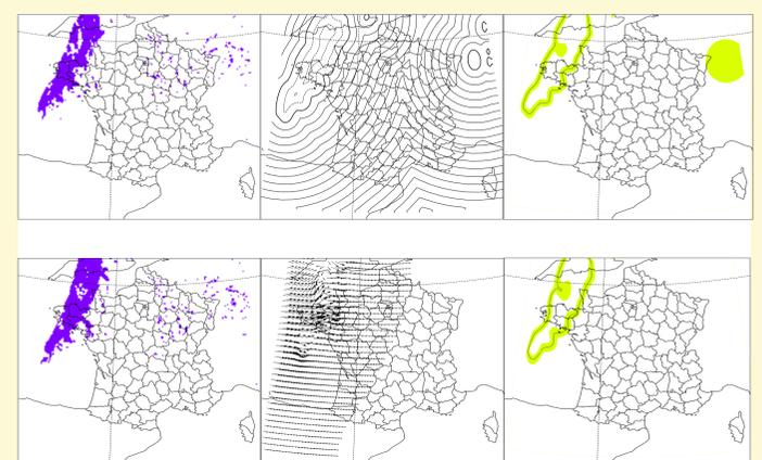
Left column: precipitation model output at 12 UTC (top) and 13 UTC (mid). Shading for precipitation in excess of 0.3 mm/h. Upper-mid panel:  $\phi$  function at 12 UTC. 2nd row-mid panel: optical flow between 12 and 13 UTC. Right column: Object tracking using the digital filter method initialized at 12UTC at the initial state (top) and 1 hour further (bottom). The solid contour stands for the mean object and the shaded area for  $\pm 2$  standard deviation of the ensemble.
