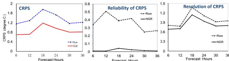
Figure 5: CRPS and its decomposition (reliability and resolution component) of 2-m temperature from raw and calibrated REPS. Verification period: 20 July to 20 August 2008
