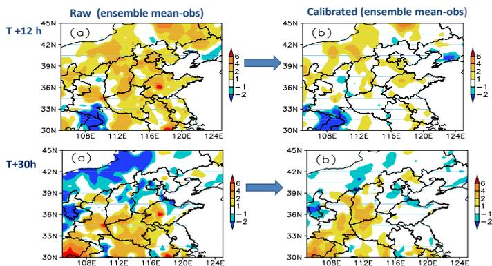
Figure 1: The raw and calibrated ensemble mean error of 2-m temperature at 12UTC 20 July 2008, +12 and +30 h lead time. Simulation domain was B08RDP common domain.
