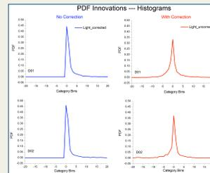
Figure 2. PDF Innovations – histograms, before and after correction. Before correction (left), the innovation vector was skewed and positively biased. After correction (right) it was normalized.
