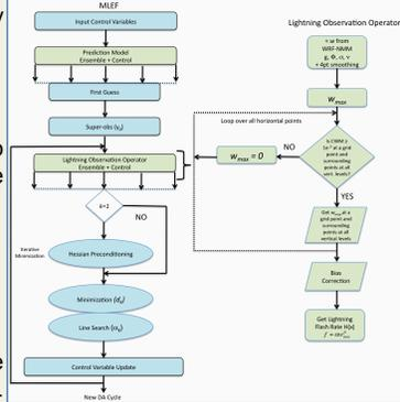
Figure 1. Flow chart of the MLEF DA system and lightning observation operator
