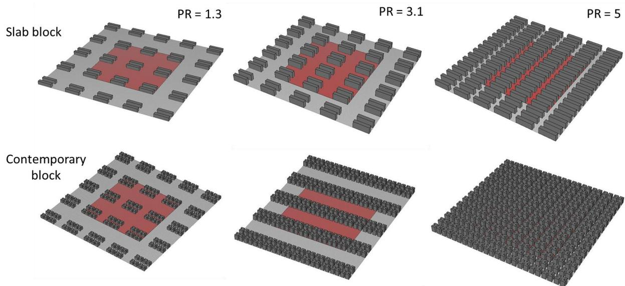
Fig. 2 Perspective view of the simulation model for the slab and contemporary blocks and the three building dispositions considered. The red area is the analysed area.
