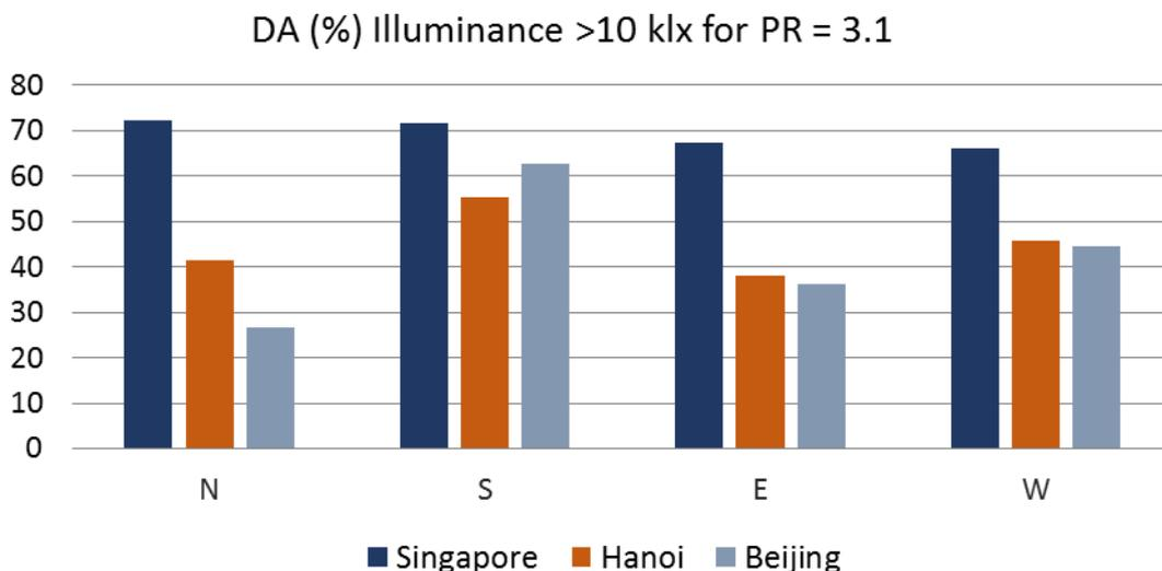
Fig. 4 Average of DA (illuminance > 10 klx) of three typologies for PR = 3.1 and the four facade orientations.
