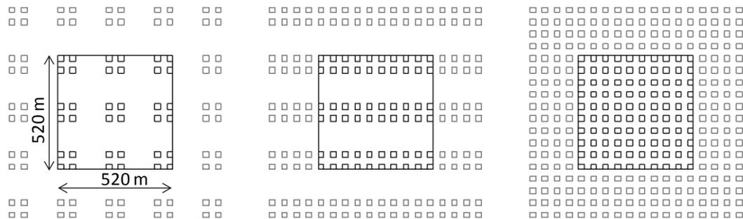
Fig. 1 Schematic of the simulation model for three building dispositions of point block typology corresponding to P-1, P-2 and P-3 cases on Table 1. The framed area is the analysed area.
