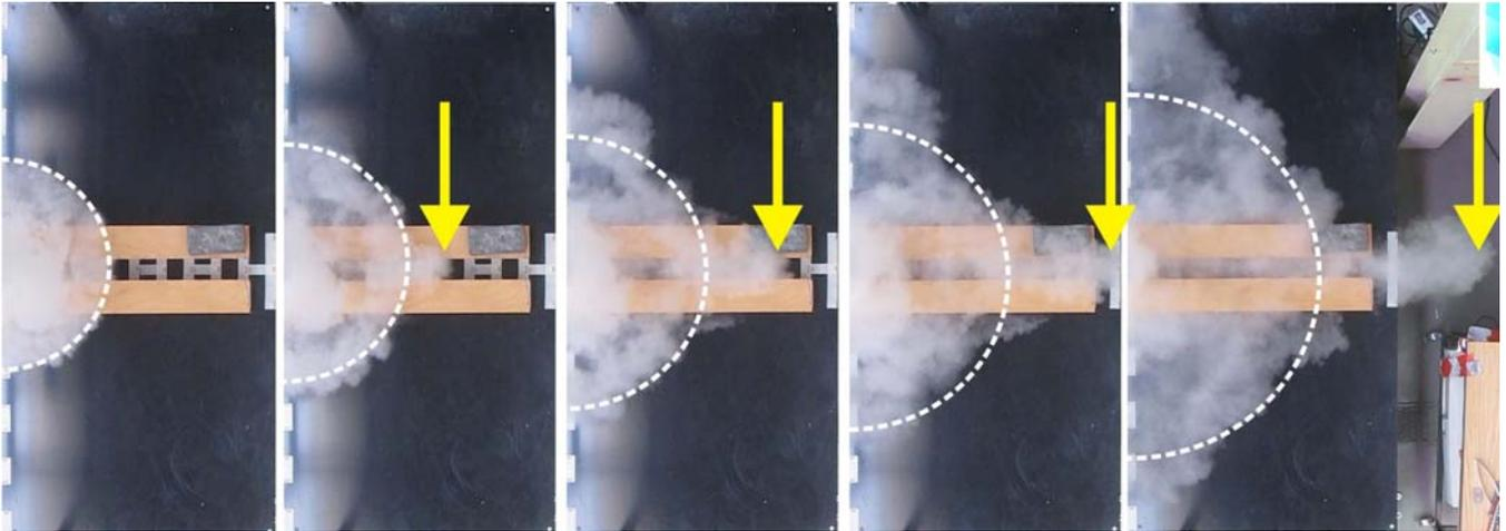
Fig. 9: Visualized downdraft (CO<sub>2</sub> with water droplets) impinges on a street canyon in a simulation experiment; the radial spreading of the primary vortex in the plane is marked with white dashed circles, the faster spreading within the street canyon is marked with yellow arrows; taken from Eggs 2015
