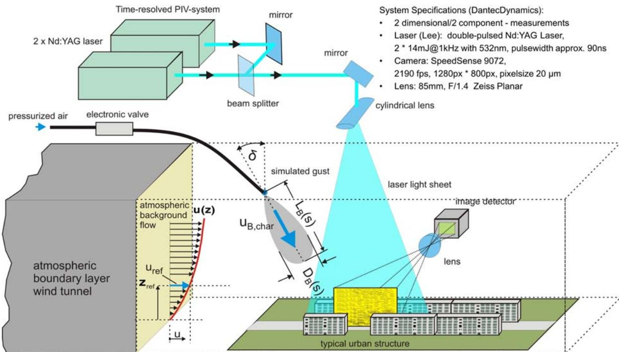
Fig. 2: Sketch of the experimental set-up consisting of boundary layer wind tunnel, gust generator, 2D-2C-TR-PIV system and urban built structure
