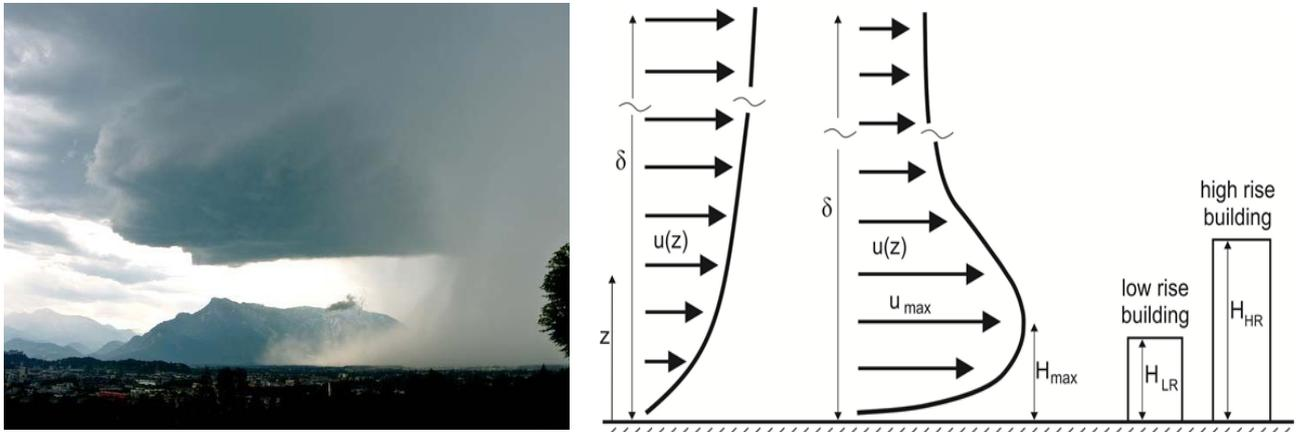
Fig. 1: *left*: Downburst over Salzburg on June 22, 2011 (Foto: Fabian Lackner) *right*: Schematic of an atmospheric boundary layer profile and the velocity profile in the outflow of a downburst
