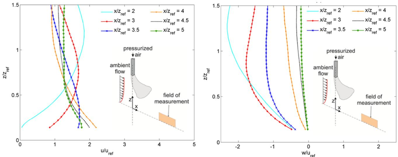
Fig. 6: Horizontal (left) and vertical (right) velocity profiles of the open terrain case - constant wall jet;  $z_{ref} = 50$  mm (i.e. 10 m in nature),  $u_{ref} = u(z_{ref})$  of the background flow
