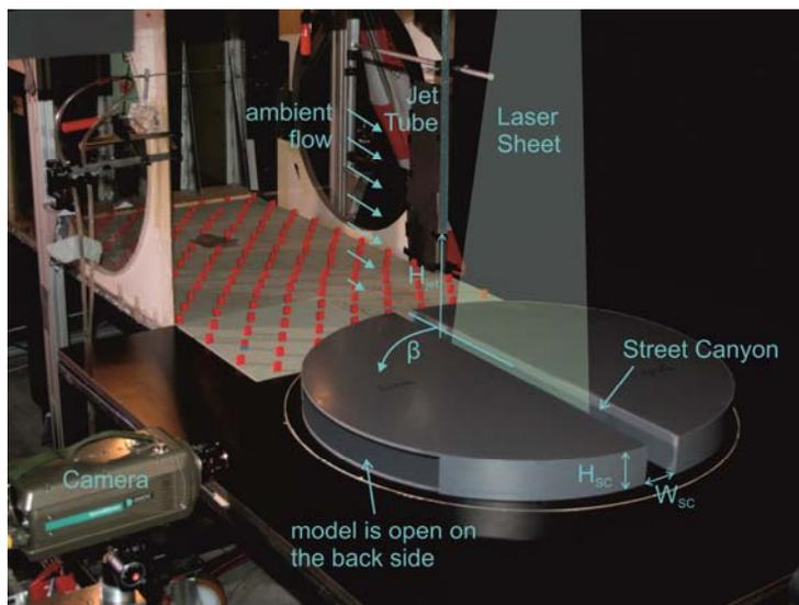
Fig. 4: Experimental setup with the street canyon
