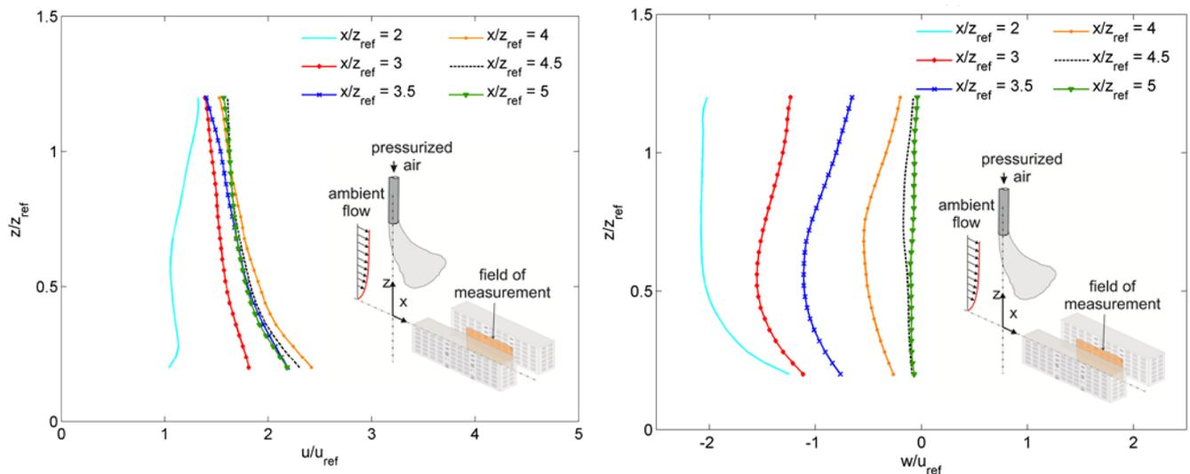
Fig. 7: Horizontal (left) and vertical (right) velocity profiles within the street canyon model parallel to the atmospheric background flow (case 2),  $z_{ref} = 50$  mm (i.e. 10 m in nature),  $u_{ref} = u(z_{ref})$  of the open terrain background flow; building height  $H = 1,5 z_{ref}$  (i.e. 15 m in nature)
