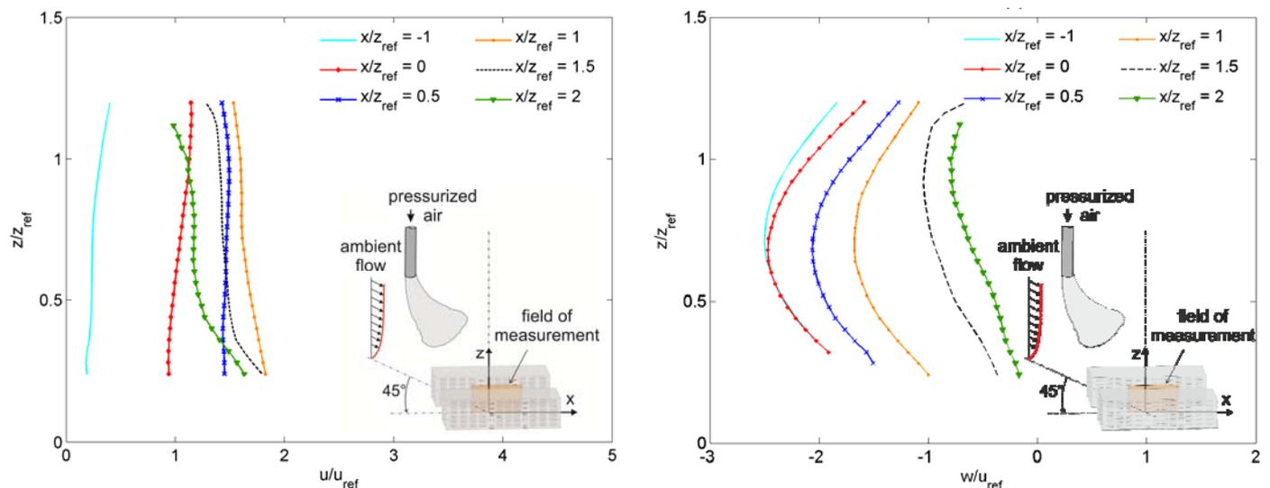
Fig. 8: Horizontal (left) and vertical (right) velocity profiles within the street canyon model with an orientation of  $\beta = 45^\circ$  (case 3),  $z_{ref} = 50$  mm,  $u_{ref} = u(z_{ref})$  of the open terrain background flow (case 1).
