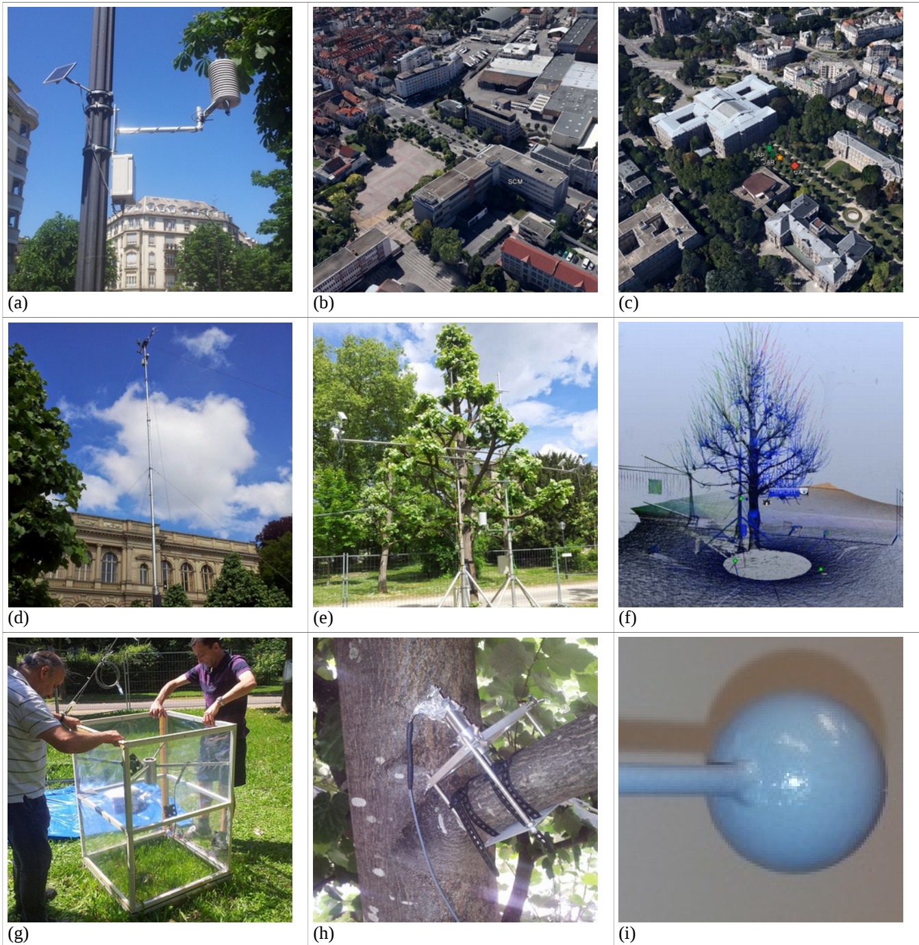
Fig. 2 (a) An example of air temperature and humidity station built in-lab, composed of an Arduino module gathering measurements from a Sensirion SHT75 probe and powered by a solar panel ; (b) Aerial view of the densely urbanized area where flux measurements are performed. The mast is set up on top of the building in the center of the picture; (c) Aerial view of the urban park of the university campus. The orange star shows the location of the 20 meters mast. (d) A view of the 20 meters mast in the urban park; (e) The linden tree equipped with a mast for air temperature and humidity profile, a mast for the PAR profile, a sap flow sensor and four infrared radiometers; (f) The same linden tree reconstructed from ground LIDAR point cloud; (g) The transpiration gas chamber to monitor the evaporation from the grass; (h) a PepiPIAF monitoring micro-metric variations of the diameter of the branches; (i) A 38 mm flat grey globe thermometer built in-lab.
