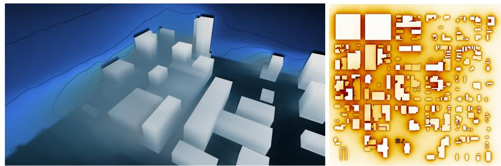
We are able to simulate and visualize volumetric scalar fields in addition to surface scalar fields. On the left, we are visualizing a simulation of energy transport in downtown Salt Lake City. The air temperature is shown as a traditional volume visualization, and clipping planes at back show the values on those planes and additional isocontours to make the data structure more easily visible.
