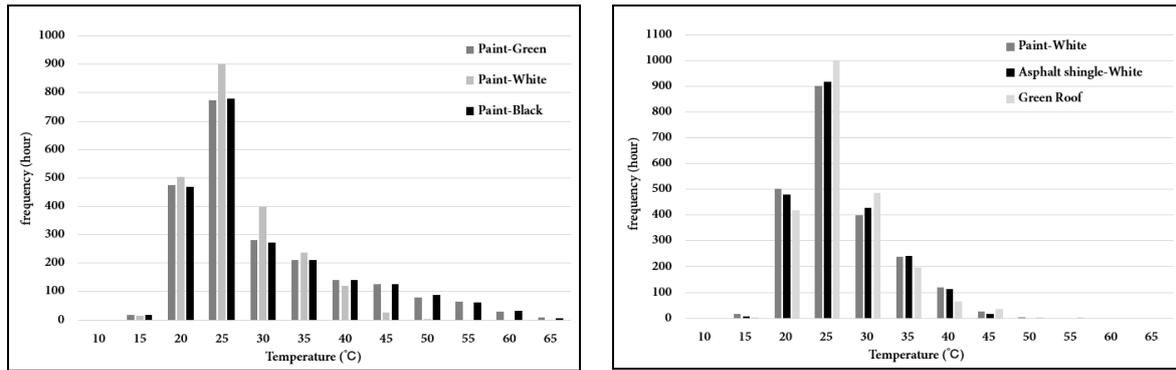
Surface temperature according to roof color.
