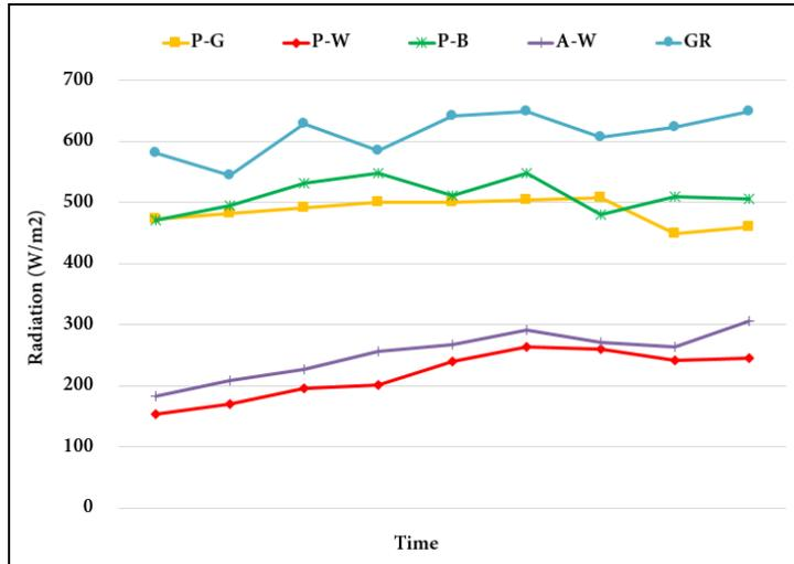
Fig 4. Changes in net radiant energy according to roof type.
