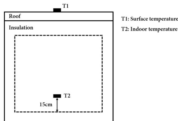
Fig 2. Temperature measurement points in the model.
