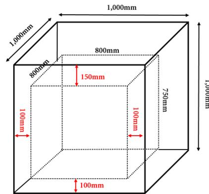
Fig 1. Blueprint for the small-scale building model.
