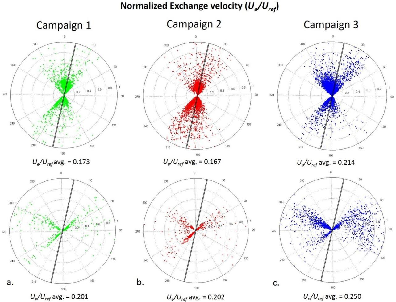
*Fig. 3 Normalized exchange velocity during Campaign 1 (a), Campaign 2 (b) and Campaign 3 (c) for parallel (top) and perpendicular (bottom) wind conditions. The black line identifies the street axis direction.  $U_e/U_{ref}$  avg. refers to the average normalized exchange velocity.*
