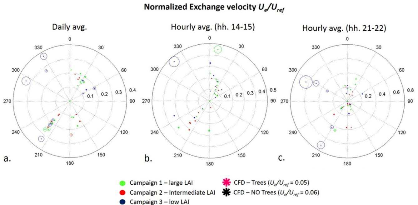
**Fig. 4** Normalized exchange velocity obtained from daily averages (a), hourly averages (hh. 14:00-15:00) during light-time (b) and 1-hour averages (hh. 21:00-22:00) during night-time (c) over the whole Main campaign. The circle size at each point indicates the standard deviation. St. dev. avg. refers to the average standard deviation for each campaign.
