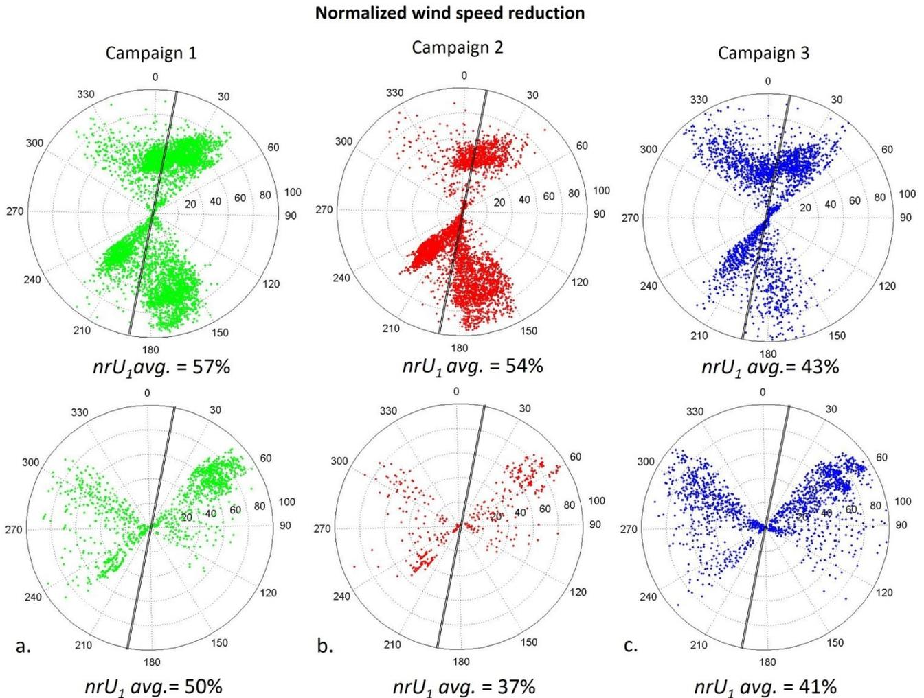
*Fig. 2 Normalized percentage reduction of wind speed during Campaign 1 (a), Campaign 2 (b) and Campaign 3 (c) for parallel (top) and perpendicular (bottom) approaching wind conditions. The black line identifies the street axis direction. nrU<sub>1</sub> avg. refers to the average wind speed reduction.*
