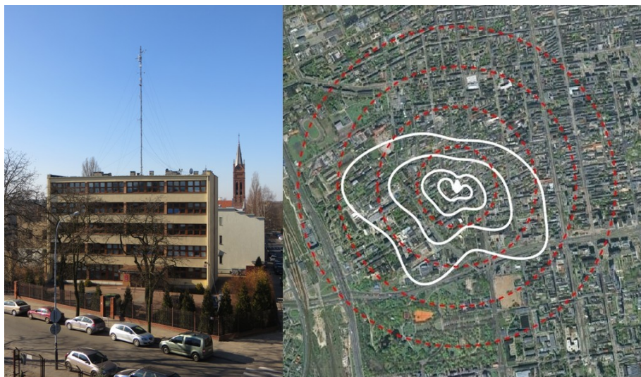
Fig. 1. FCO_2 and FCH_4 measurement site (left) and aerial photo of site surroundings in the western part of Łódź center (right). White lines indicate source area with probability P = 25, 50, 75 and 90\% calculated for unstable conditions in the period July 2013 – April 2015. Red dotted lines indicate 250, 500, 750 and 1000 distances from the measurement site.
