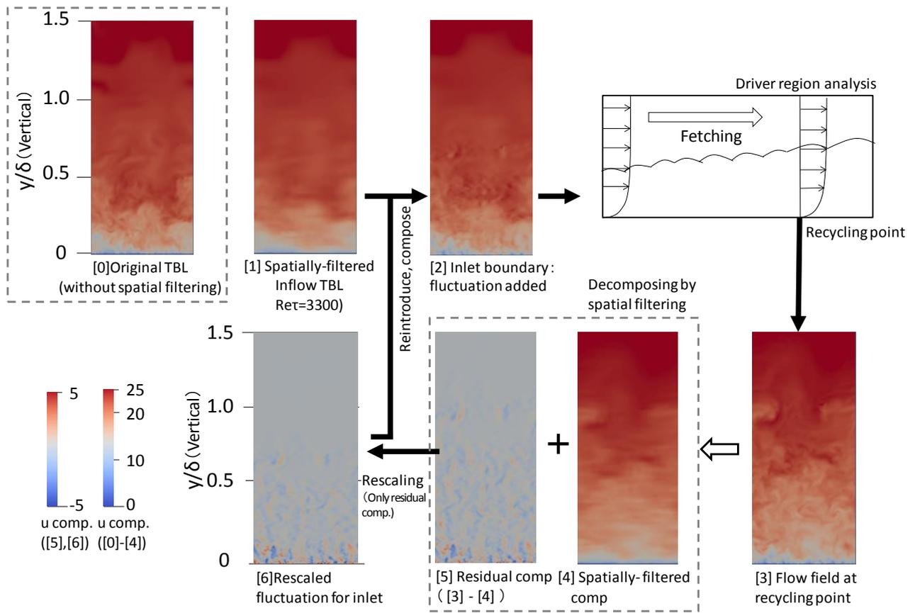
Fig.4. Adding process of high frequency fluctuation in the computed result
