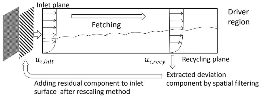
Fig.1. Driver region calculation for adding high-frequency fluctuation to spatially-filtered inflow
