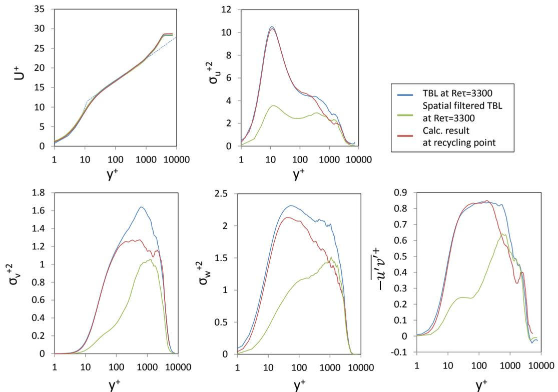
Fig.5. Computed results of turbulent statistics: Does the high frequency fluctuation recover?
