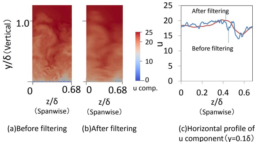
Fig.3. Inflow condition: Spatially-filtered turbulent boundary layer ( $\text{Re}\tau=3300$ )
