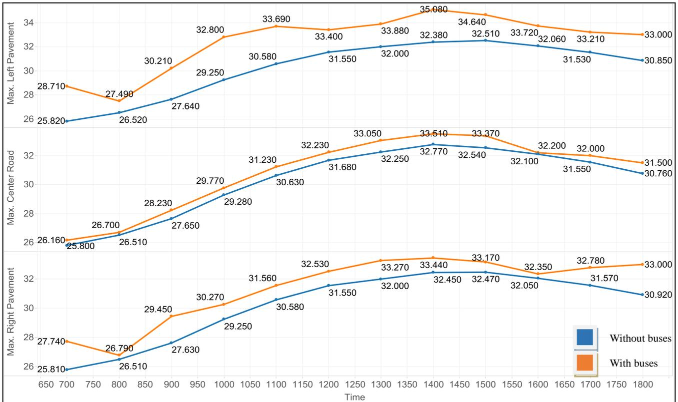
Fig. 8 Point measured air temperature with and without bus heat at 1.5m in the urban canyon for point and slab typologies for both parallel and perpendicular wind flow.
