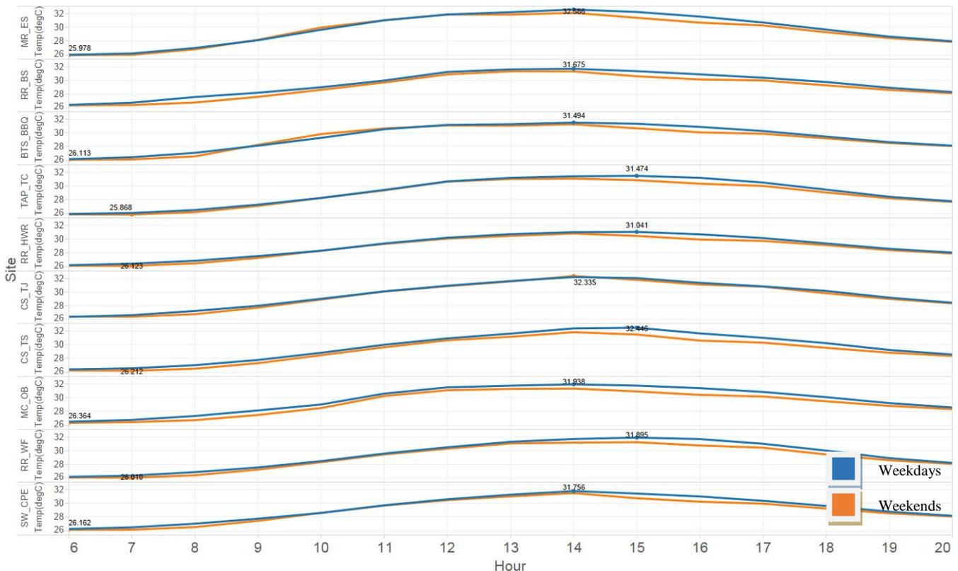
Fig. 2 Weekdays and weekends (February 2014) air temperature at 3.5m above ground (MR\_ES=Maxwell Road\_Edge of Site, RR\_BS=Robinson Road\_Bus Stop, BTS\_BBQ=Boon Tat Street\_Barbeque Stalls, TAP\_TC=Telok Ayer Park\_Trees Canopy, RR\_HWR=Robinson Road\_High Height-to-Width Ratio, CS\_TJ=Cecil
