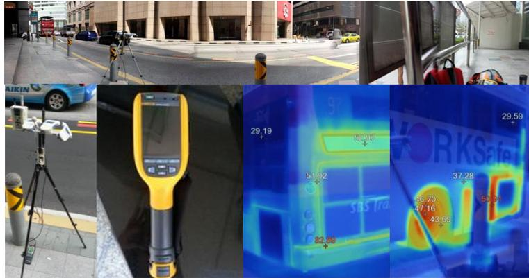
Fig. 3 CBD urban canyon roadside measurement (above), measurement equipment (below left) and infrared images of bus surfaces (below right).
