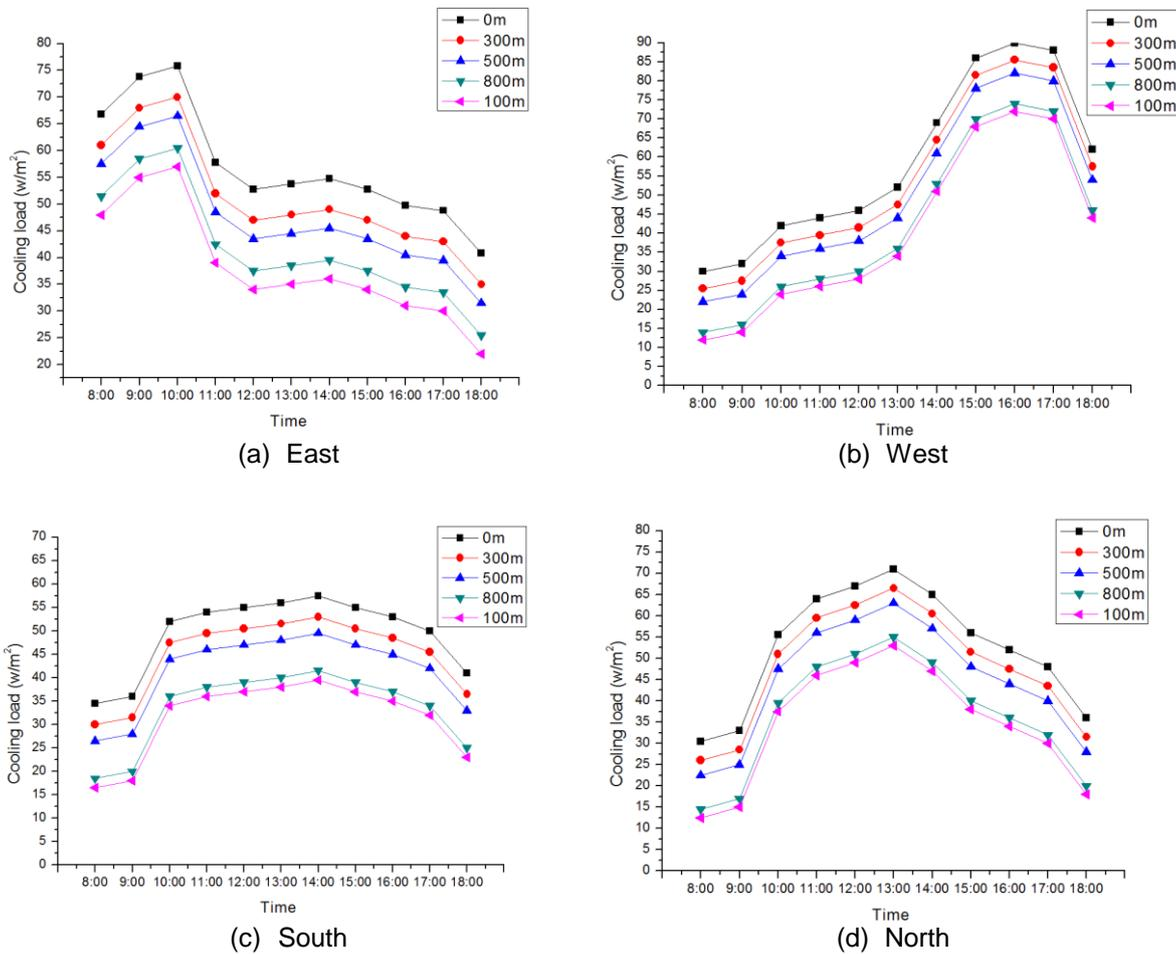
**Fig12 Variation of hourly cooling load with height**
