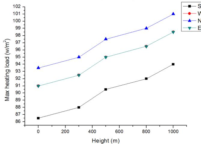
**Fig13 variation of design heating load with height**
