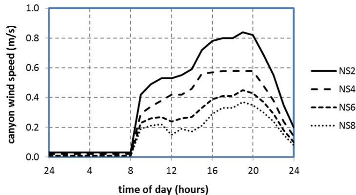
Fig. 2: Wind speed at pedestrian height (1.5m) in a N-S street canyon 15m wide flanked by buildings of different heights (2-8 storeys).
