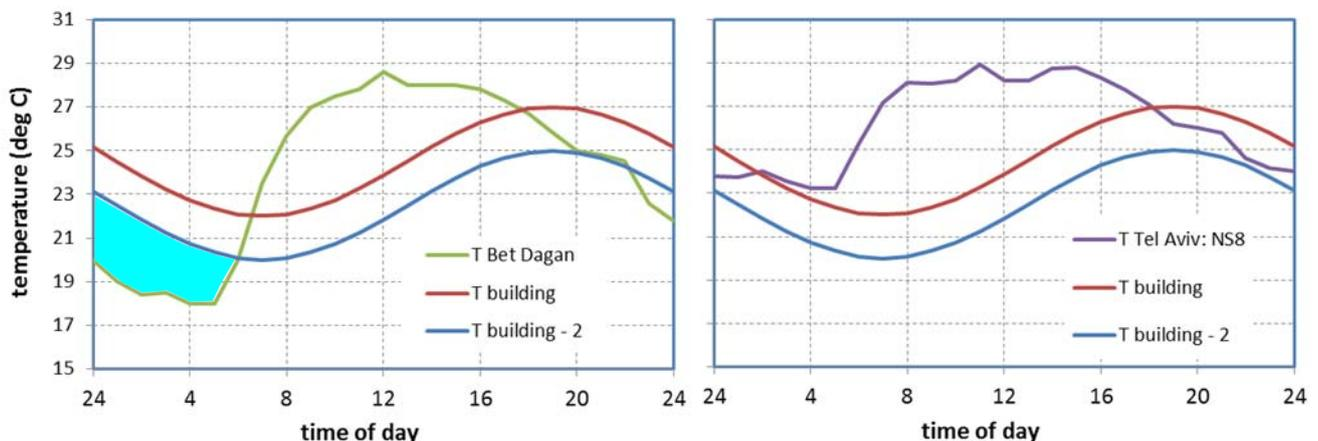
Fig. 3: Climate cooling potential on a typical day in July. On the left – CCP calculated for an exposed building at Bet Dagan. On the right – the CCP for a building in a street with 8-storey buildings, using air temperature generated by CAT.
