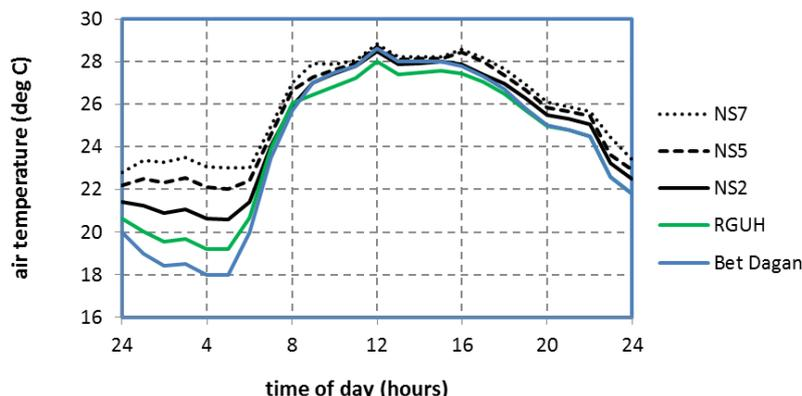
Fig. 1: Dry bulb temperature at the Bet Dagan weather station, simulated effects on air temperature of vegetation and water bodies (referred to here as 'rural geometry-urban hydrology', RGUH) and predicted temperatures for a N-S street canyon flanked by buildings of 2, 5 and 7 storeys.
