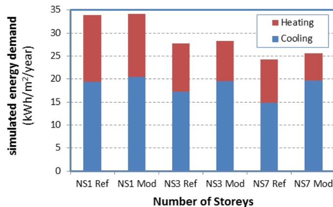
Fig. 4: Simulated energy demand for heating and cooling buildings on a N-S canyon, for building heights of 1, 3, and 7 storeys. Buildings simulated with TMY data from the reference site at Bet Dagan are referred to as 'ref' and those simulated with TMY modified to account for urban site conditions according to different density scenarios are referred to as 'mod'.
