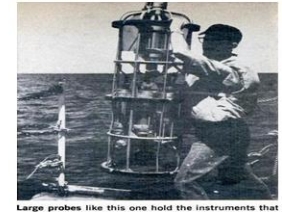
Large probes like this one hold the instruments that automatically measure salinity, temperature, and depth as they are lowered to the ocean bottom.
