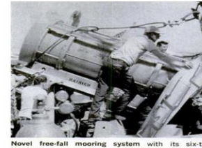
Novel free-fall mooring system with its six-ton clump anchor took a bit of handling when loaded aboard the station ship Rainer at Gulfport, Miss.
