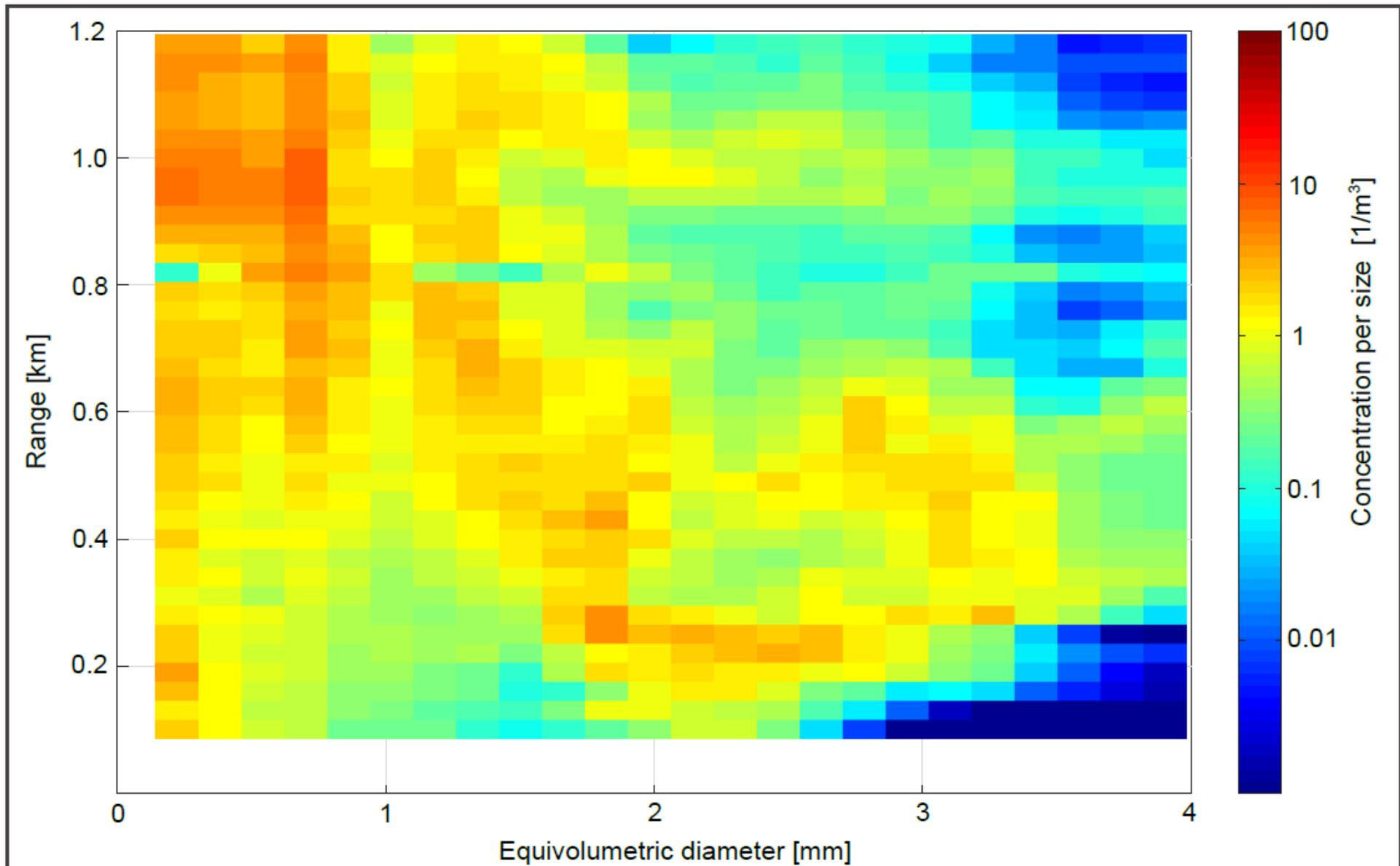
**Fig. 8. DSD profile retrieved with the optimal estimation procedure.**
