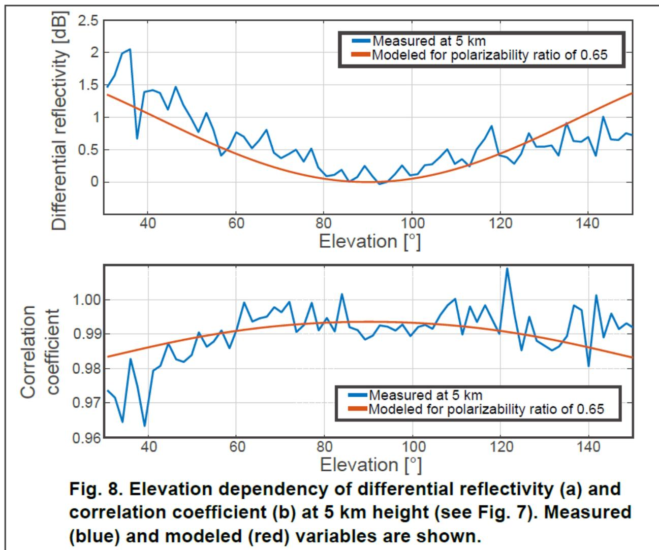
**Fig. 8. Elevation dependency of differential reflectivity (a) and correlation coefficient (b) at 5 km height (see Fig. 7). Measured (blue) and modeled (red) variables are shown.**
