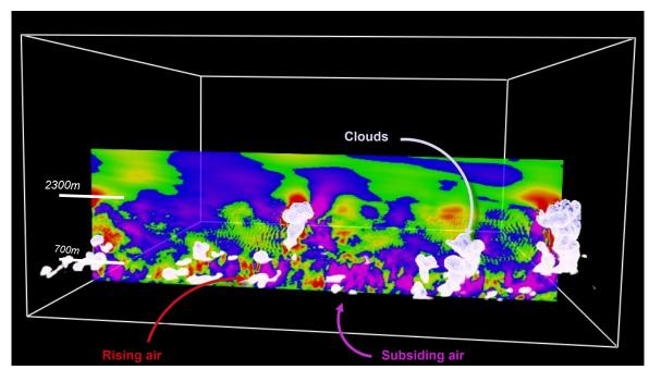
Δx=25m Large-Eddy Simulation, RICO test-case
