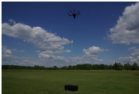
Tethered drone carrying a target simulator
