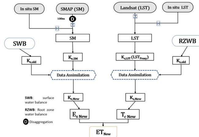
**figure 2.** Schematic diagram of the assimilation approach.  $E_{s,New}$ ,  $T_{c,New}$ ,  $K_{e,New}$ ,  $K_{s,New}$  are the updated evaporation, transpiration, evaporation and stress coefficient after assimilation, respectively.  $K_{e,old}$  and  $K_{s,old}$  are  $K_e$  and  $K_s$  before assimilation, respectively.
