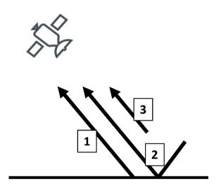
$$Tb_p = T_{surf} \times \epsilon_p \times e^{-\tau(0,H)/\mu} + T_{atm}^{\downarrow} \times (1 - \epsilon_p) \times e^{-\tau(0,H)/\mu} + T_{atm}^{\uparrow}$$
