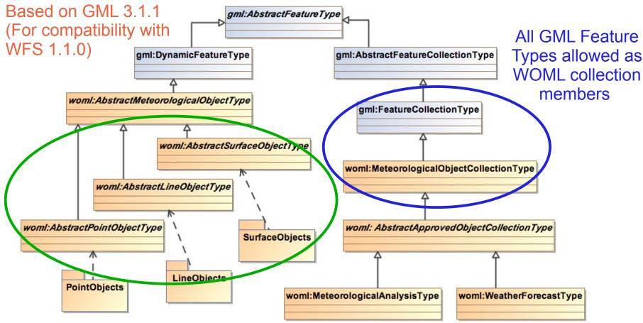
Geometry-based typing: Extended types can at least be properly geo-located
