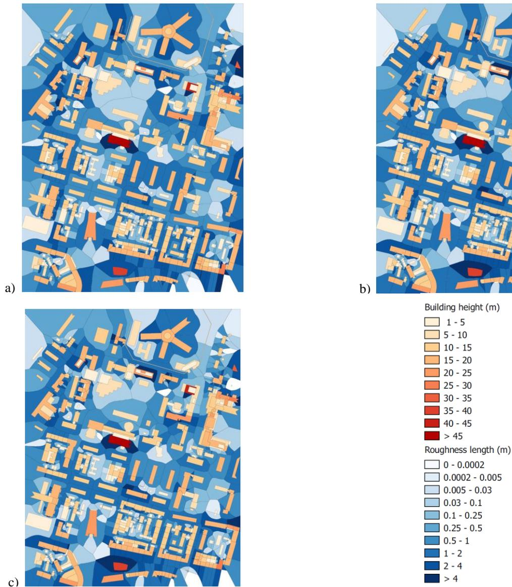
*Fig. 5 Estimation of roughness after Bottema (1997) for different wind directions a) 90° b) 225° c) 360° for a specific area in the northern part of Freiburg (Meteorological Urban Climate Station Freiburg is located on highest building)*
