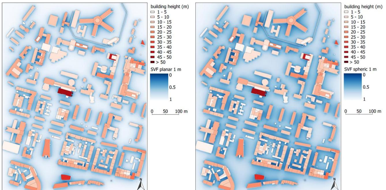
Fig. 4 Sky View factor for a part of Freiburg (Meteorological Urban Climate Station Freiburg is located on highest building, left: planar SVF, right: spheric SVF) with resolution 1x1 m at height of 1 m
