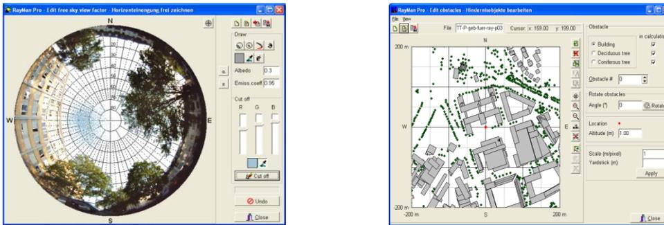
Fig. 1 Input possibilities in RayMan (left: fish-eye, right: geometrical obstacles).
