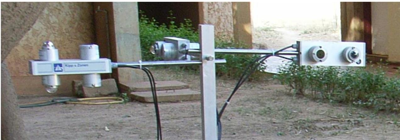
Fig. 1. Equipment to monitor the short- and longwave fluxes in six directions
