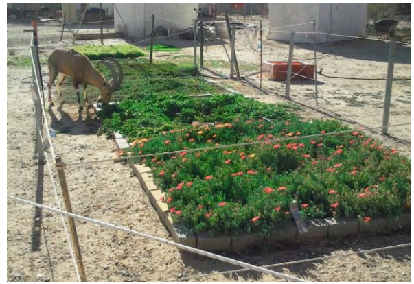
Figure 8. Experimental plots planted with six types of succulent and other species, for measurement of albedo and surface temperature, as input for the calculation of ITS in urban spaces.
