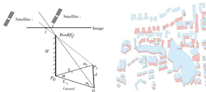
*Fig. 1 The method of building's span and height identification
