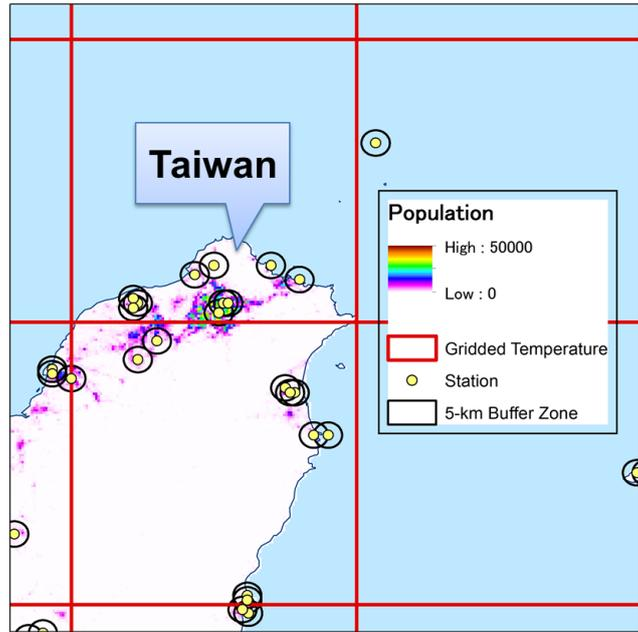
Fig. 3 Example of the stations used in BEST and its bounding temperature grids. Circles represent the 5-km buffer zones. Colored contours represent the LandScan population data.
