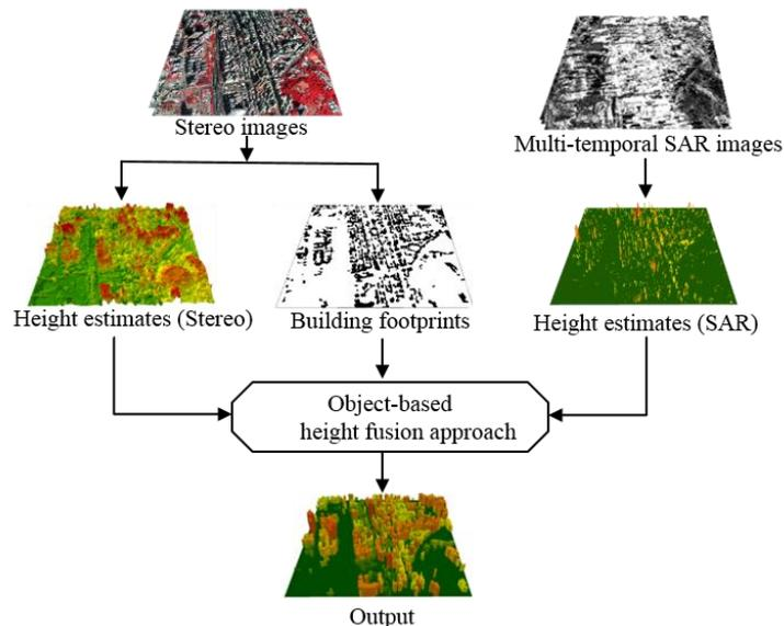
Figure 1. Procedure of the proposed approach for 3D building extraction
