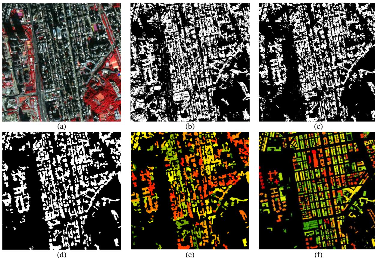
Figure 2. 3D building extraction with the proposed approach. (a) High-resolution satellite image. (b) Preliminary extracted objects using the object-oriented classification method. (c) Filtered result by removing the objects with low heights. (d) Extracted building footprints. (e) The extracted building footprints and building heights with the proposed approach. (f) Actual 3D building information for comparison.
