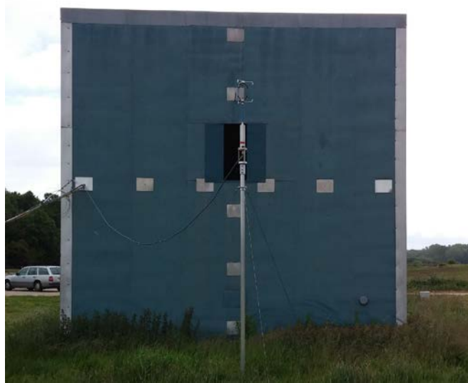
Fig. 3 The isolated cube and the sonic anemometer in front of the 0.4 m 2 vent.
