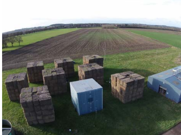
Fig. 1 Drone photograph of the straw cube array, array masts, the instrumented cube (blue) and the surrounding areas. The camera is facing to the North-West.
