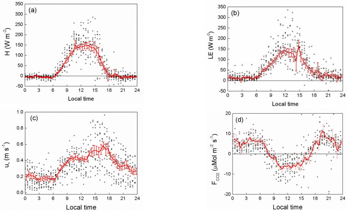
**Figure 7:** Diurnal evolution of turbulent vertical fluxes of (a) Sensible heat, (b) Latent heat, (c) friction velocity and (d) CO<sub>2</sub> observed during the 1<sup>st</sup> Campaign carried out the MRSP in February of 2013. Observations carried out in the PM IAG.
