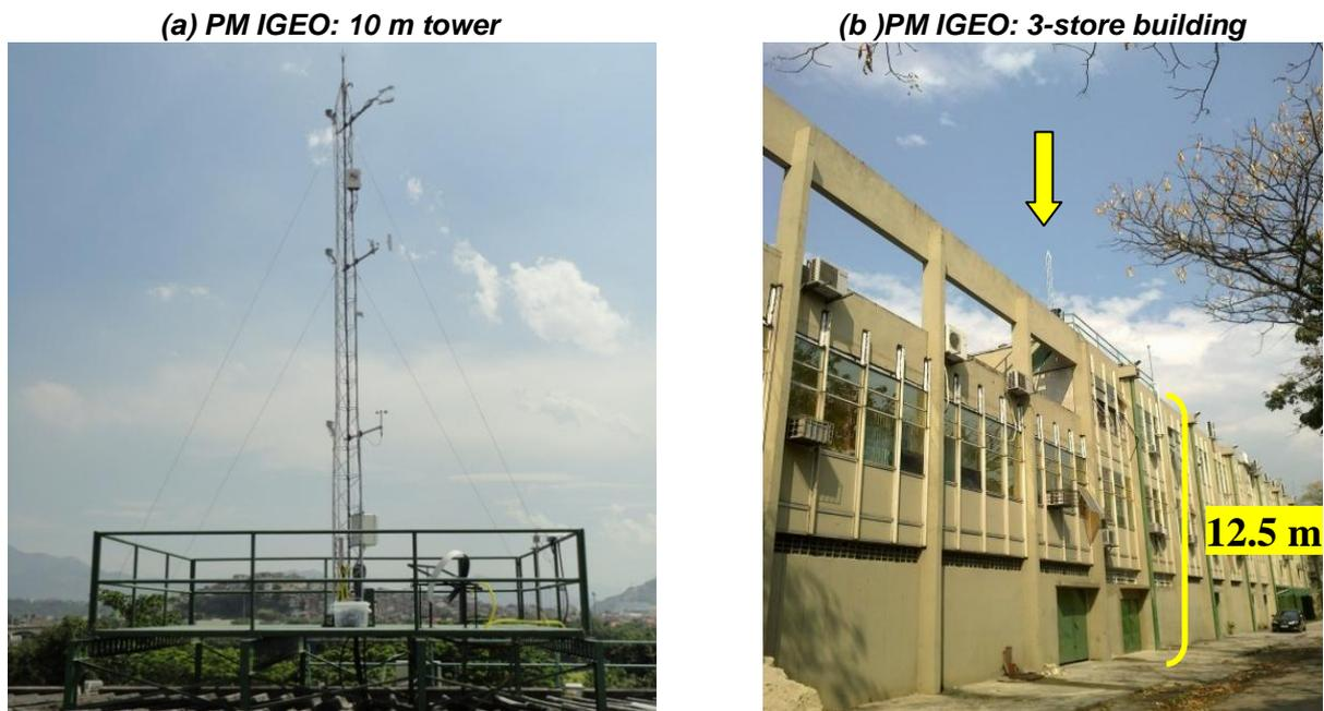
**Figure 6.** Micrometeorological platform of IGEO (PM IGEO) located in the top of a 3-store building at the University of Rio de Janeiro Campus at Fundão Island: (a) 10-m tower, (b) 3-store building .
