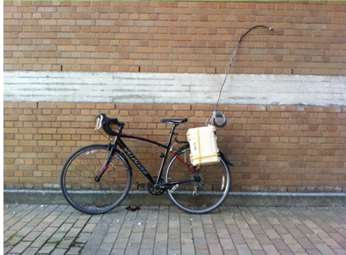
Figure 5: Sensor installation on (a) vehicle and (b) bike. The sample tubes reach approximately 2m height.
