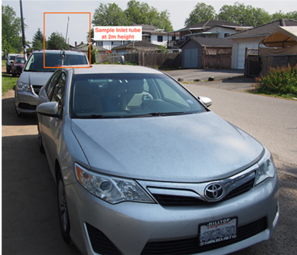
Figure 5: Sensor installation on (a) vehicle and (b) bike. The sample tubes reach approximately 2m height.
