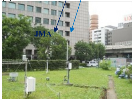
Fig.1. (a) The Otemachi meteorological enclosure at the Tokyo Regional Headquarters, Japan Meteorological Agency. The upper side is almost the north. (b) The main thermometer (at the start and end points of the indigo arrow), called "JMA", and the central anemometer (the aqua arrow) in the enclosure. (c) The extra thermometer (the pink arrow), called "Field", with the other anemometer (the green arrow).
