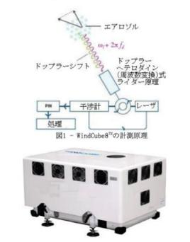
Fig. 1 Measuring Principle of Doppler Lidar System (DLS)
