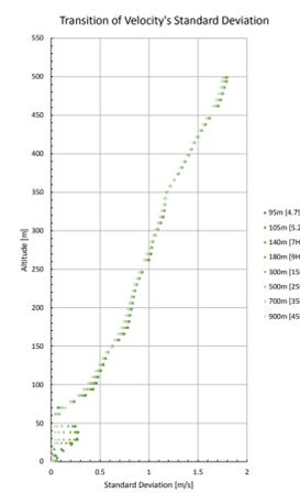
Fig. 10 Standard deviation of fluctuated profiles
