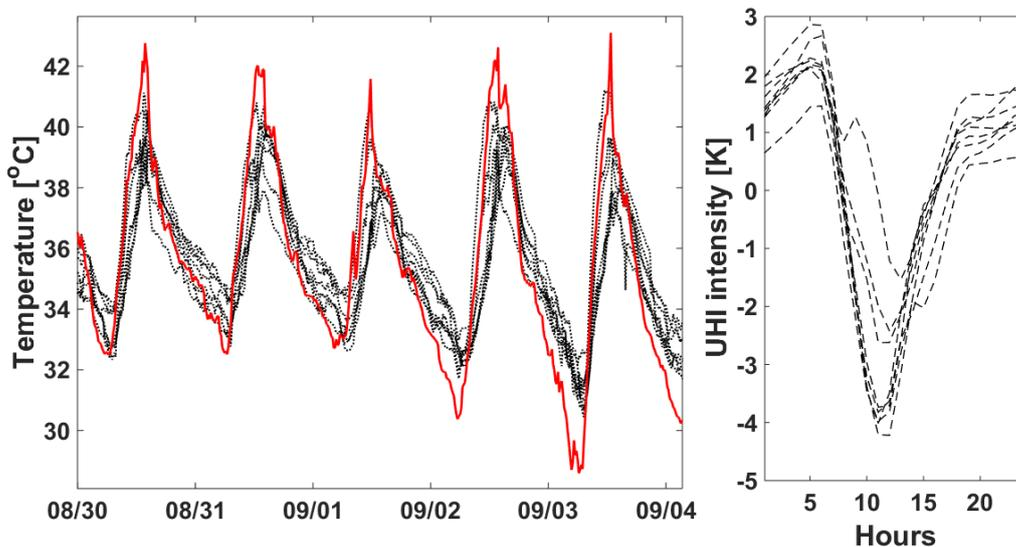
Fig. 6 Urban (black) and open desert (red) temperature (left), and average diurnal cycle of UHI intensity (right) measured at Masdar Institute from August 13<sup>th</sup> to September 31<sup>st</sup> 2011
