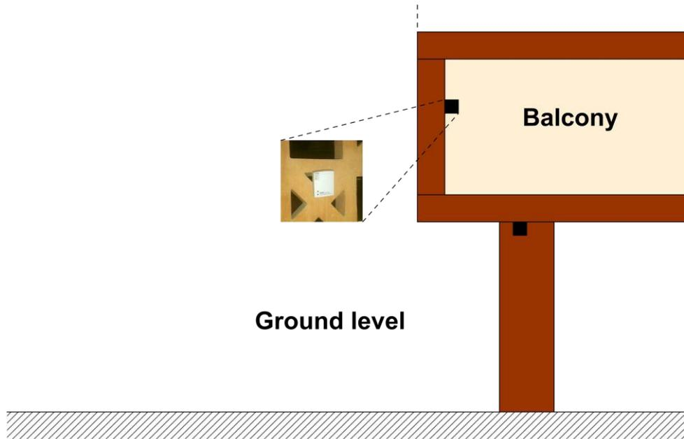
Fig. 3 Typical HOBO logger (dark square) installation
