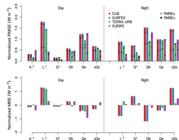
**Figure 4:** Normalized RMSE (top row) and MBE (bottom row) for modelled daytime (left panels) and nighttime (right panels) fluxes. All models simulations are performed using the REF namelist. The systematic and unsystematic normalized RMSE are depicted with respectively crosses and dots (top panels).
