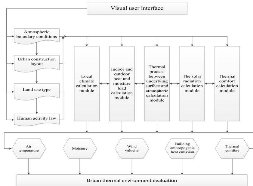
Fig.2 Structure diagram of UDC model
