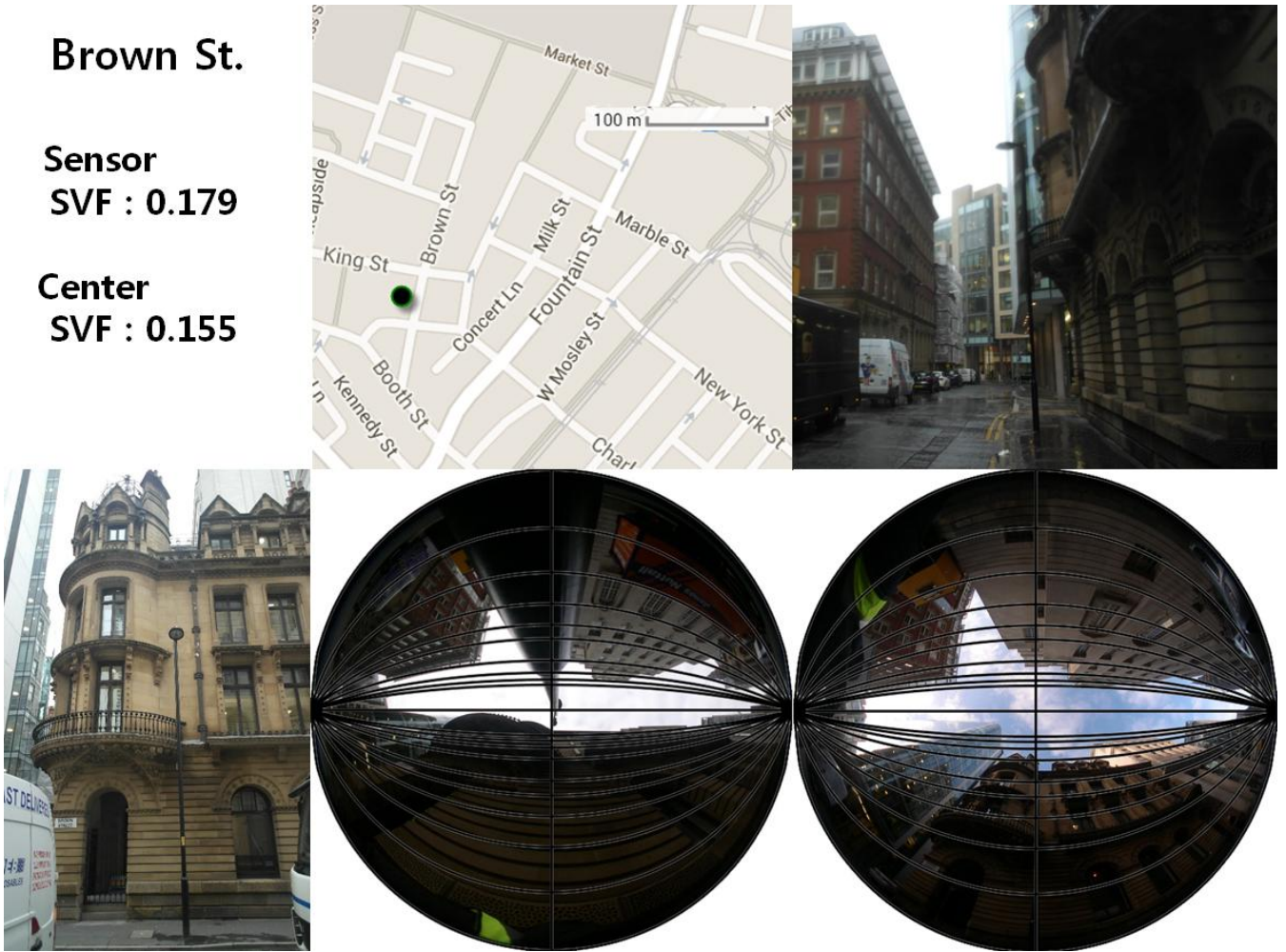
Fig. 4 Picture of fish-eye lens and SVF for sensor and center of road in Manchester center
