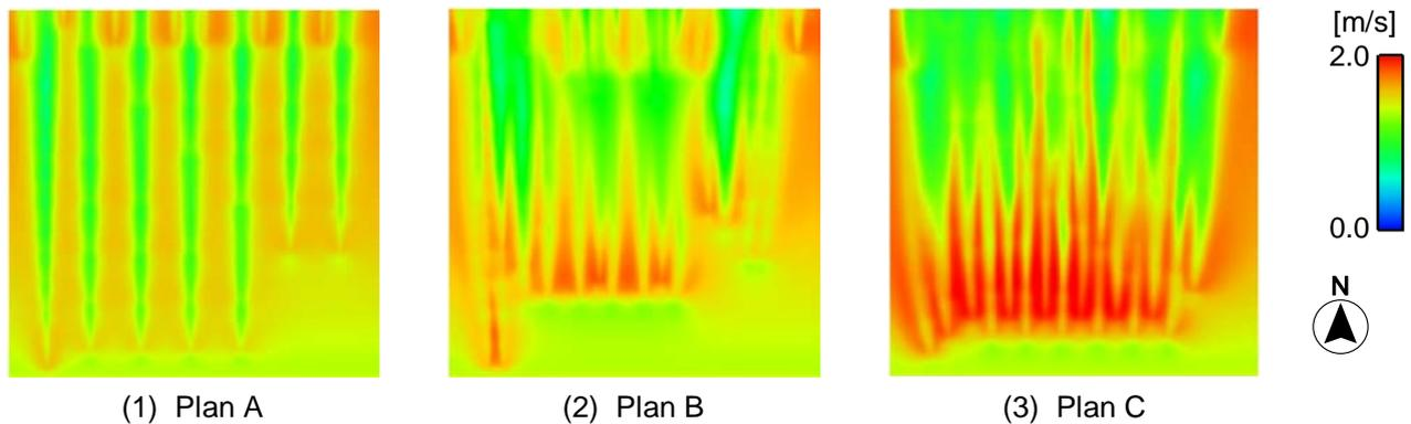
Fig.6 Horizontal distribution of wind velocity at the height of 1.25m
