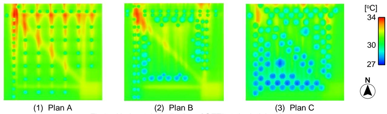
Fig.8 Horizontal distribution of SET\* at the height of 1.25m
