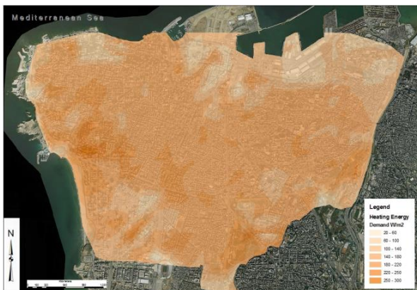
Figure 7. Heating energy demand simulations for Control Run across Beirut on 01-Feb. 1200UTC
