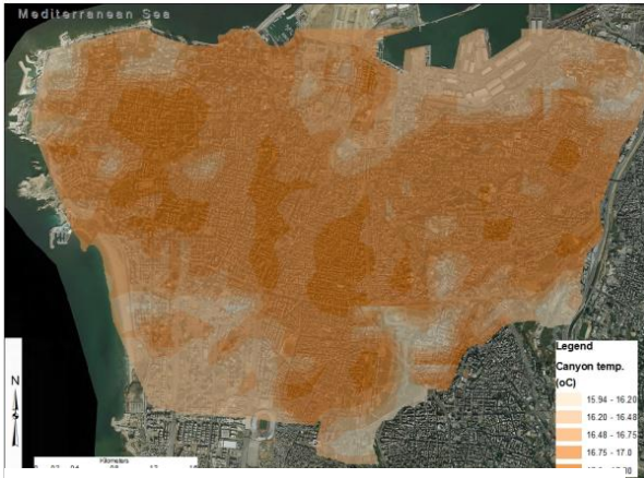
Figure 3. Canyon temperature simulations for Control Run across Beirut on 01-Feb. 1200UTC
