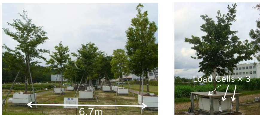
Fig. 1 Photos of farm field (left) and measurement of tree weight using load cells (right).
