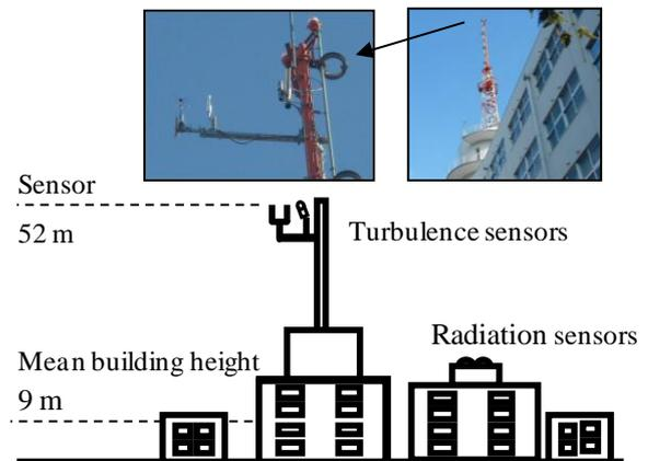
Fig. 2. The measurement tower.
