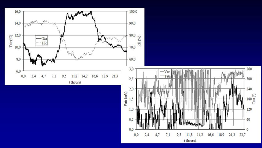
Measured outdoor air temperature, air relative humidity, air velocity and wind direction, for a typical winter day.
